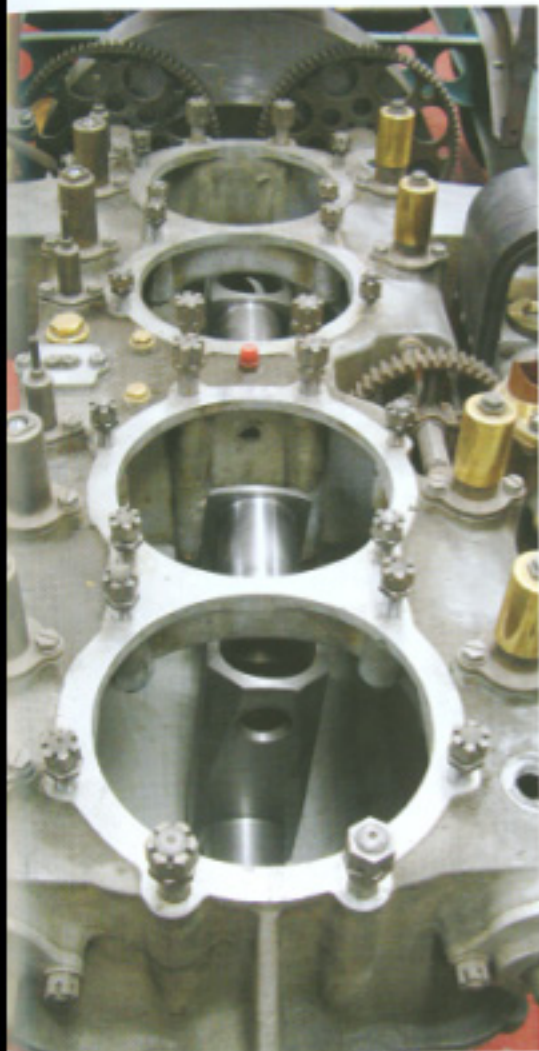
Above: Two pairs of cylinders were mounted on a cast aluminum crankcase. The hollow crankshaft was forged. Right: The gear set illustrates the level of quality that went into the racers.
