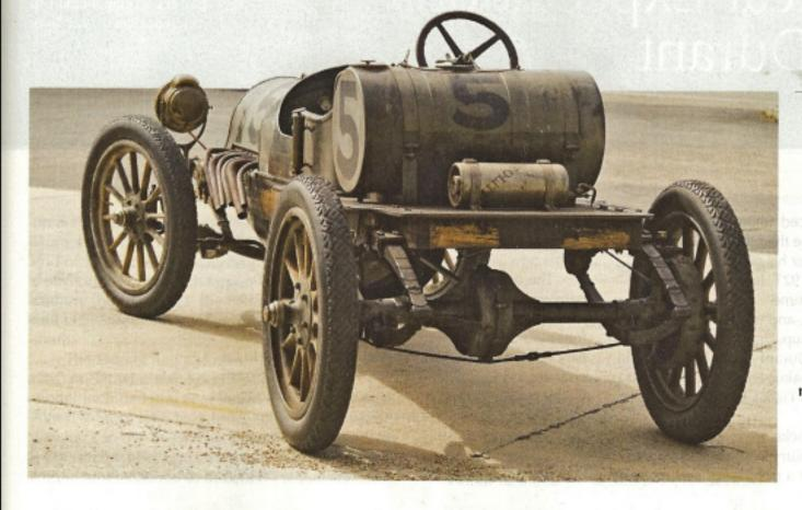
Small Prest-O-Lite acetylene generator snuggles in behind a massive gas tank. No water is needed for the air-cooled engine. Rear deck held two spare tires in race trim, with toolbox. It's hard to imagine what it took for Hamlin to crush an identical, massive differential. Hamlin and Carris finally won the race in 1912 after coming second to the same winning Kissel team again in 1911.
