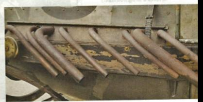
Even in 1910, they knew this was something special, and reporters remarked on the spectacular engine. The hybrid D engine in an H chassis benefits from Franklin's improved shrouding to cool the engine, plus the massive front opening to admit extra air at high speeds.
