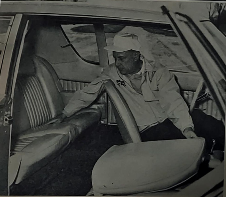
Wide doors and full width rear seat, left, aid easy use of this area for extra passengers. The front seats fold flat, have latex foam padding. Built-in roll bar is high tensile steel tube fastened to frame and padded into head liner.
