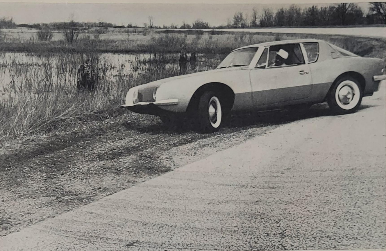
Stable on soft gravel or hard pavement, the Avanti has quick steering response, can be turned in 33 foot circle.
