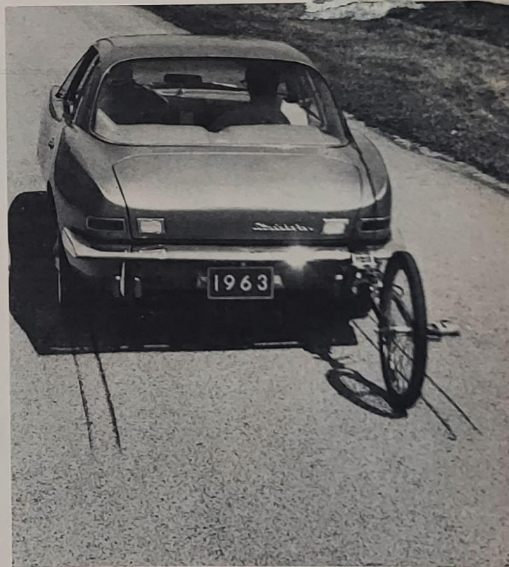
Twin traction differential gives both wheels good bite while accelerating on any type of slick or dry pavement.
