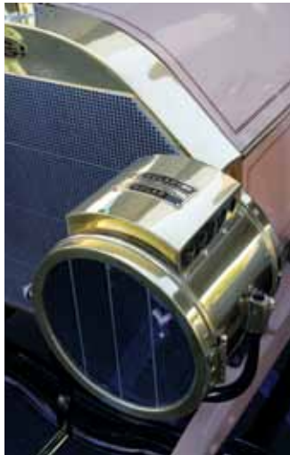
For driving after dark, the Mercedes had two acetylene headlights, plus two oil-fueled running lights and one taillight.
